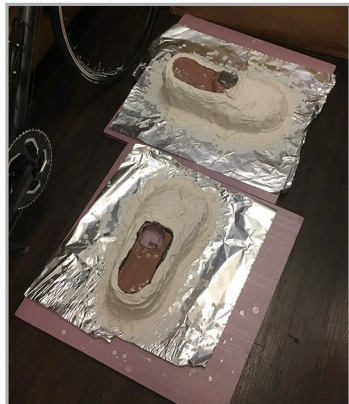
Thickened VytaFlex 50 mold covered in plaster bandages.
