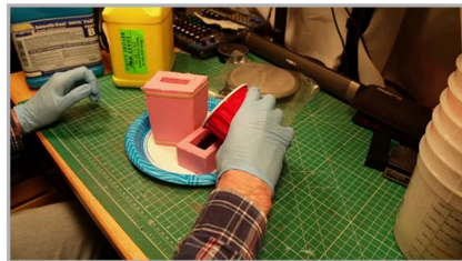
Pouring resin into dump molds to cast the skinny and wide bandolier boxes.
